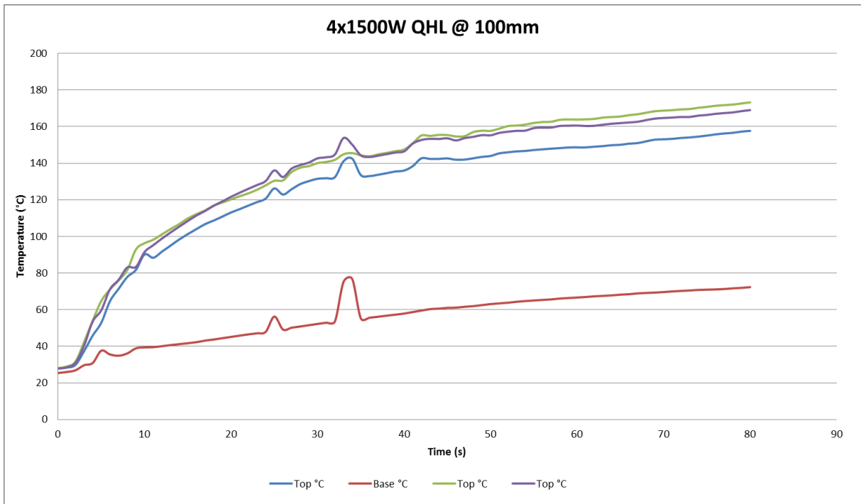
Figure 4. Time temperature curve for the composite a distance of 100mm from the 1.5kW QHL tubes
