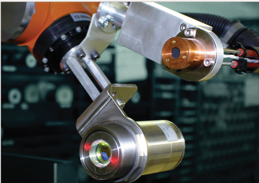
The heart of The Herschel is a Schmidt-Boelter radiant heat flux sensor. This specialized sensor uses IR transparent glass, specialized material and temperature sensor systems to measure the IR heat impinging upon a target that is less than 1 millimeter in size.
