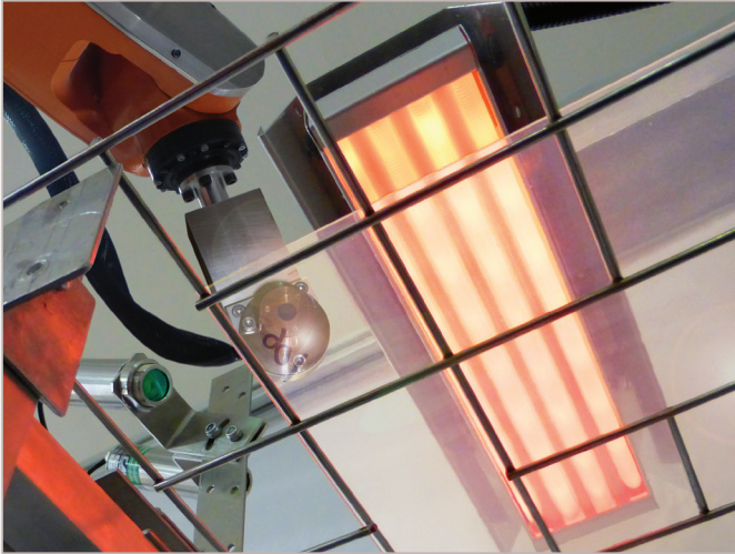
The Herschel software programs have been written to generate 3d images having facilitated the positioning of the heat flux sensor anywhere and in any position in front of heaters and heater assemblies
