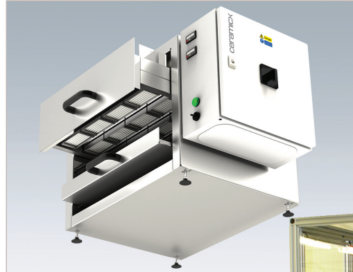
8kW bench top test unit supplied with 3 interchangeable infrared heating plattens consisting of Ceramic, Quartz and Quartz Tunsten/Halogen Tubes.
